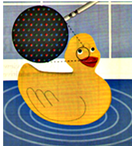
On a TV screen or computer monitor, however, the entire gamut of colors is created from a black screen by triads of red, green and blue phosphors, which vary in intensity according to the strength of the electron beam that hits them.
